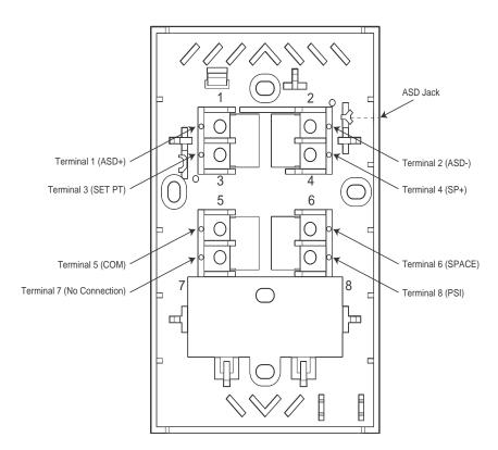
Figure-3 Base Plate Terminal Identification.
