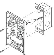
2 X 4 Electrical Box Pigtail Mounting.
