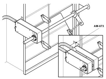
Figure-4 Mounting Multiple Actuators.
