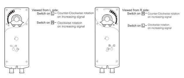
Figure-3 Rotation Switch Settings.
