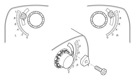
Figure-5 Adjusting Stop Block for Limited Rotation.
