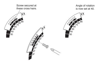
Figure-6 Securing the AM-689 Rotation Limiter.
