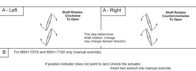
Insert hex wrench into manual override. Crank the actuator so the indicator points to 0°. Lock the actuator.
