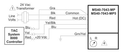
Figure-1 Proportional Control of System 8000 Room Temperature Controller Application of MS40-7043-XXX SmartX Actuator.
