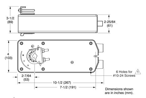
Note: These are not through holes. Use hardware supplied in Schneider Electric approved AM kits.
