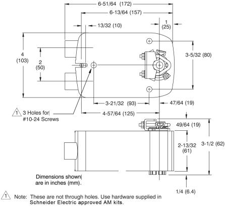
Figure-9 MS40-7043 Spring Return Damper Actuator Dimensions.
