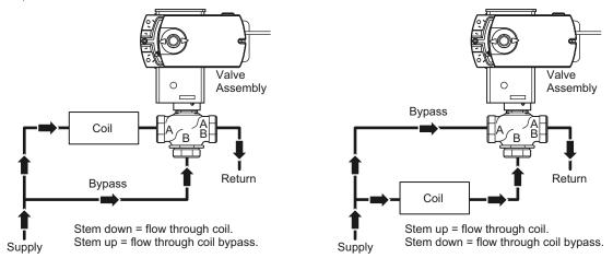
Figure 4. Typical piping of 3-Way mixing Valve for Control of Heating or Cooling Coil
