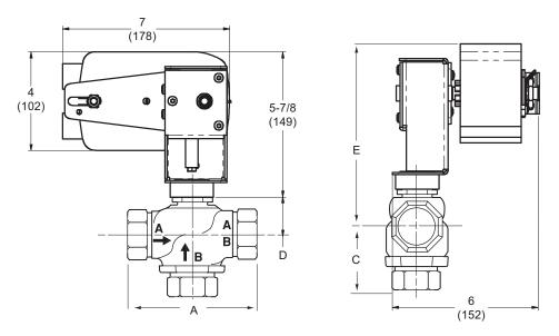
Figure-23 Mx40-704x with 1/2" to 2" 3-Way Globe Valve With AV-611 Linkage.
