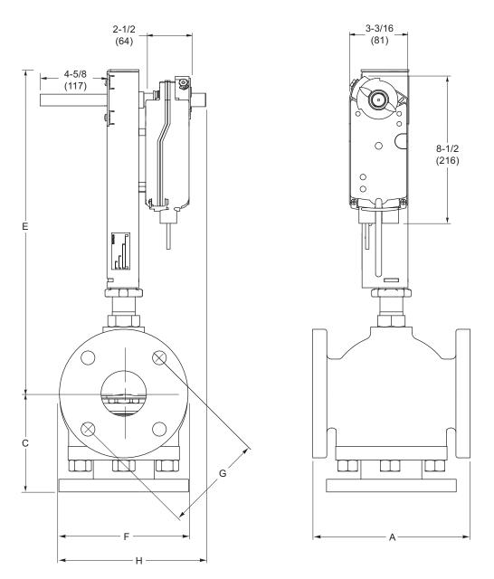
Figure-18 Mx41-6153 with 2-1/2" to 4" Flanged 3-Way Globe Valve With AV-607-1 Linkage.
