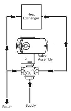
Figure 6. Typical 3-Way Diverting Valve Piping
