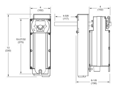
Figure-21 Mx41-6343 Actuator/Linkage Assembly With AV-609-1 Linkage.
