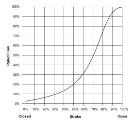
Figure 1. Typical Modified Equal Percentage Flow Characteristics
