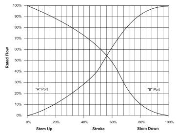
Figure 2. Typical Flow Characteristics
