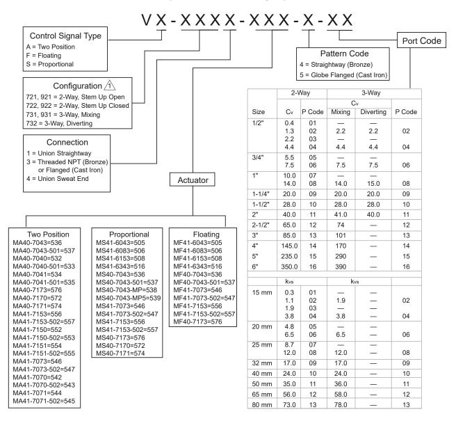
The configuration of the valve assembly determines the valve stem position and flow, as shipped from the factory. See the table below.
