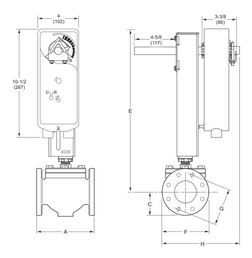
Figure-32 Mx41-715x or Mx41-707x with 2-1/2" to 4" 2-Way Flanged Globe Valve with AV-607-1
