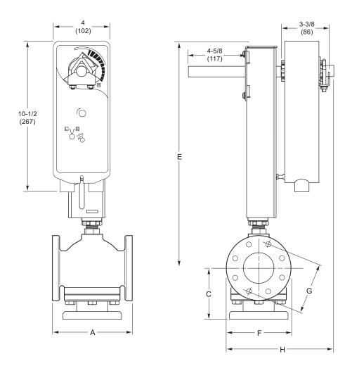
$\label{thm:prop:signature} \mbox{Figure-33 Mx41-715x or Mx41-707x with 2-1/2" to 4" 3-Way Flanged Globe Valve With AV-607-1 Linkage.}$
