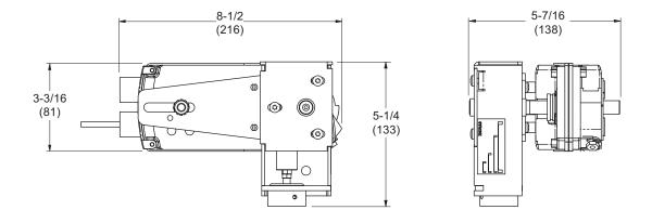
Figure-14 Mx41-6153 Actuator/Linkage Assembly with AV-611 Linkage.
